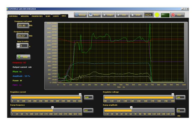
There is an inserted function for **recording data** – frequency, output current, phase, amplitude and power. Select the duration of the record in the field "**time to write**" – in seconds. The recording starts by START of the generator and ends when the selected time to write is finished. After recording is finished, when the button read is pressed, the data from generator is uploaded in the Labview software and is visualized graphically.
